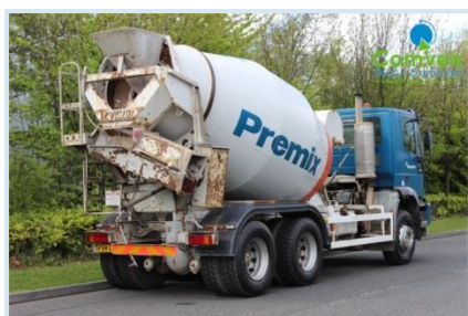
Figure 5 - Example 3 axle mixer
